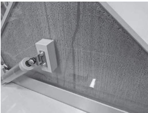
図3 槽壁面の付着液滴
