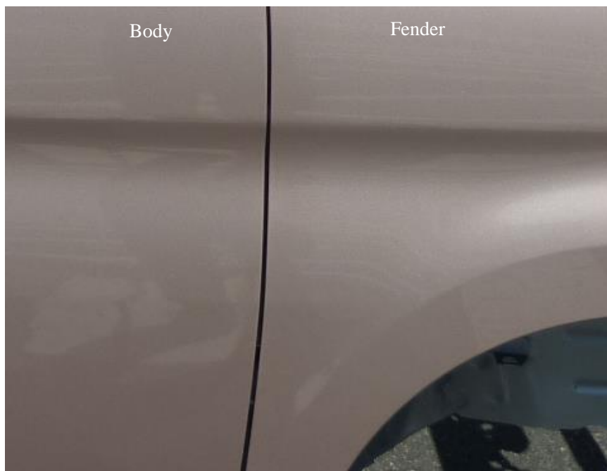
Fig.2 Color matching example (In the mass-production stage)
